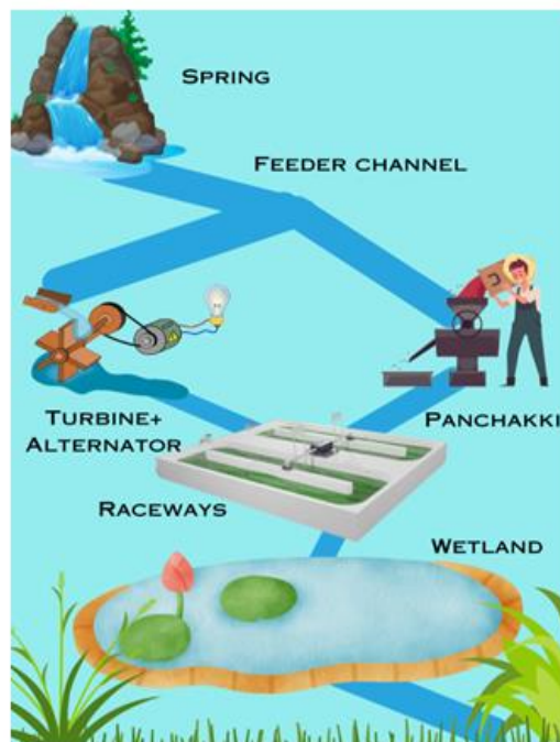
Fig. 6 Running water system innovated to include a turbine and panchakki receiving water directly from the water source and an artificially constructed wetland at the exit of the model to discharge water with comparatively less organic load
